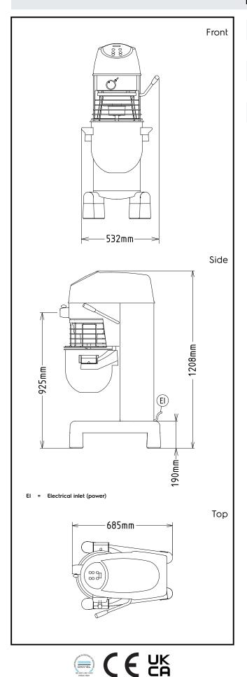
Electric Supply voltage: 200-240 V/1N ph/50/60 Hz Electrical power max: 1.01 kW Capacity: Performance (up to): 6 kg/Cycle Capacity: 20 litres
